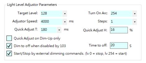
**Target Level:** The lux level (or the sensor value) to be meet. When the sensor value is higher than the Target Level \* (100% + Hysteresis), it will dim the Dimming Target to lower lumen. When the sensor value is lower than the Target Level \* (100% - Hysteresis), it will dim the Dimming Target to higher lumen.
