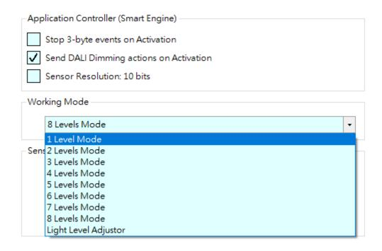
**Stop 3-byte events on Activation:** When checked, it will not send 103 events. **Send DALI Dimming actions on Activation:** When checked, it will send 102 dimming commands.
